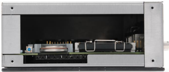
Fig. 16 Open side view with Reset button, battery and Cfast (image may vary)
