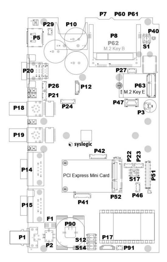
Fig. 10 Board Layout RSL81 Baseboard Top Side
