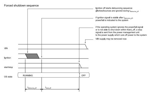
Fig. 25 Shutdown timing diagram
