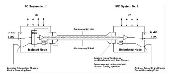
Fig. 29 Isolated communication link
