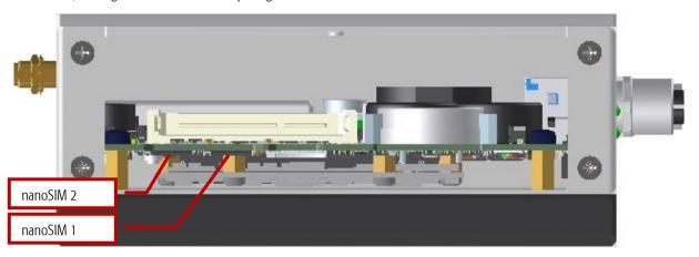
Fig. 27 SIM card installation
