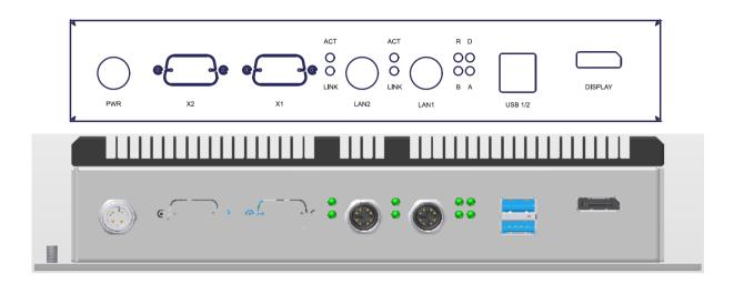
Fig. 2 Front Connections IPC/RSL81I20-A151E
