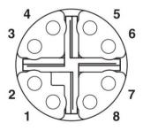
Fig. 15 M12 D-coded Female Pinout (front view)
