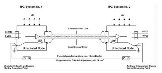
Fig. 30 Non isolated communication link with common chassis potential
