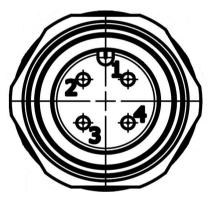
Fig. 20 M12 A-coded Male Pinout (front view)
