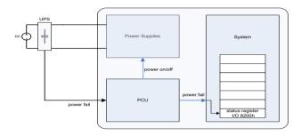
Fig. 21 Typical power fail application
