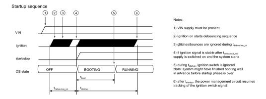
Fig. 24 Startup timing diagram
