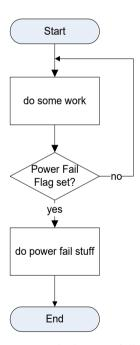
Fig. 22 Typical power fail flow
