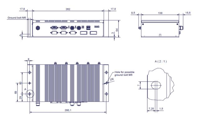
Fig. 34 Mechanical Outline Enclosure IPC/RML81I20-R152E
