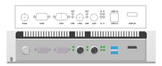
Fig. 4 Front Connections IPC/RSL81I20-R152E
