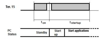
When the vehicle starts, the LH edge ("LH"- switch on, "HL" - switch off) at terminal 15 initiates the startup process. The time period  $t_{on}$  provides security for contact debouncing at the ignition switch; afterwards, the actual startup process is initiated. The embedded box PC boots, its applications start. During  $t_{startup}$ , the status of terminal 15 is not evaluated.
