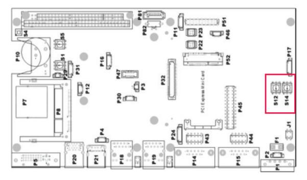
To use the remote on/off feature the position of switch S12 must be rotated to position "1".
