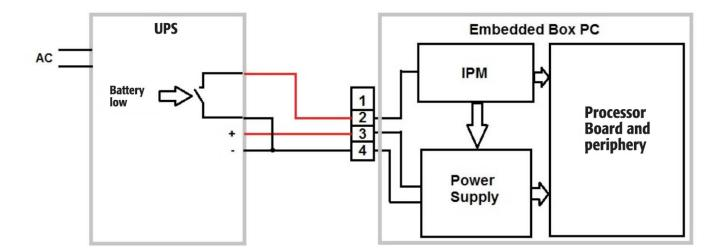
The embedded box PC must be configured to power fail mode as per the manual (coding switch S12 to position 2, coding switch S14 to position 0). To initiate the power fail if the uninterruptible power supply does not provide sufficient power, you must set the signal on pin 2 to low or bridge pin 2 and pin 4.
